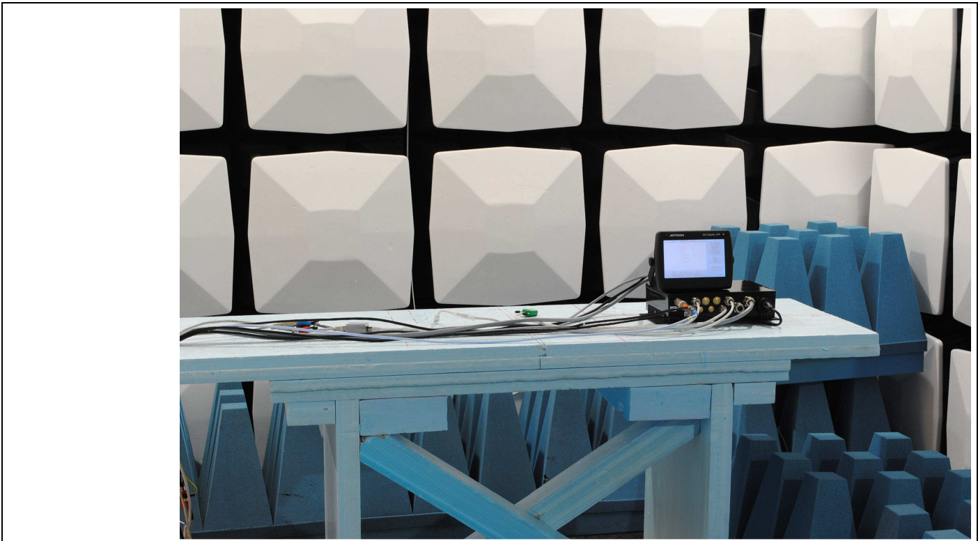
Notes: Test set-up for Radiated RF Field immunity
