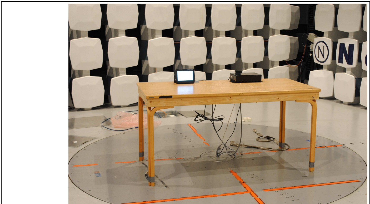
Notes: Test set-up for Radiated Disturbance 30-2000 MHz
