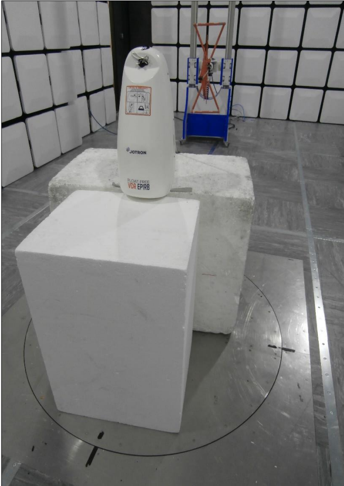
Figure 8 - Test Setup - 30 MHz to 1 GHz
