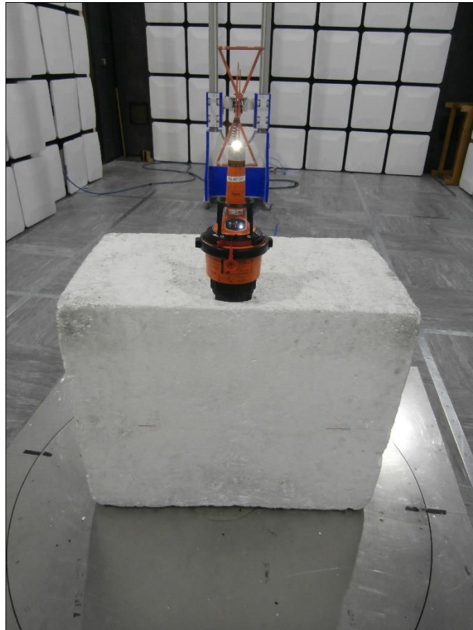
Figure 21 - Test Setup - 30 MHz to 1 GHz
