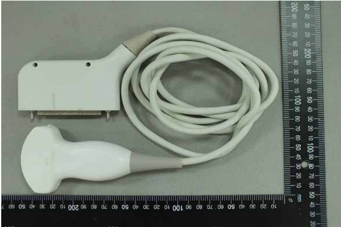
Transducer – 2 (Model No.: L115A, Supplier: Qisda Corporation)
