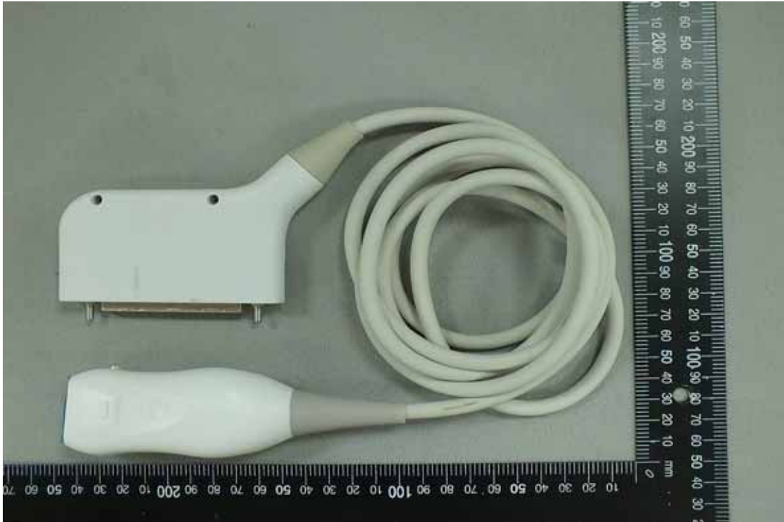
Transducer – 4 (Model No.: E94A, Supplier: Qisda Corporation)
