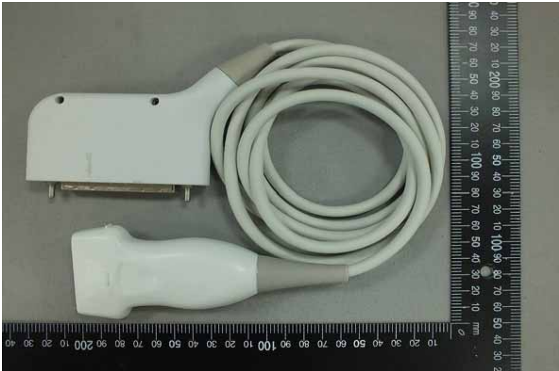
Transducer – 2 (Model No.: L115A, Supplier: Qisda Corporation)
