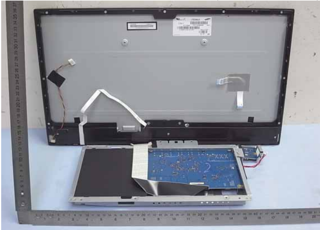
Figure 9 Internal View (Removed Shielded Case)
