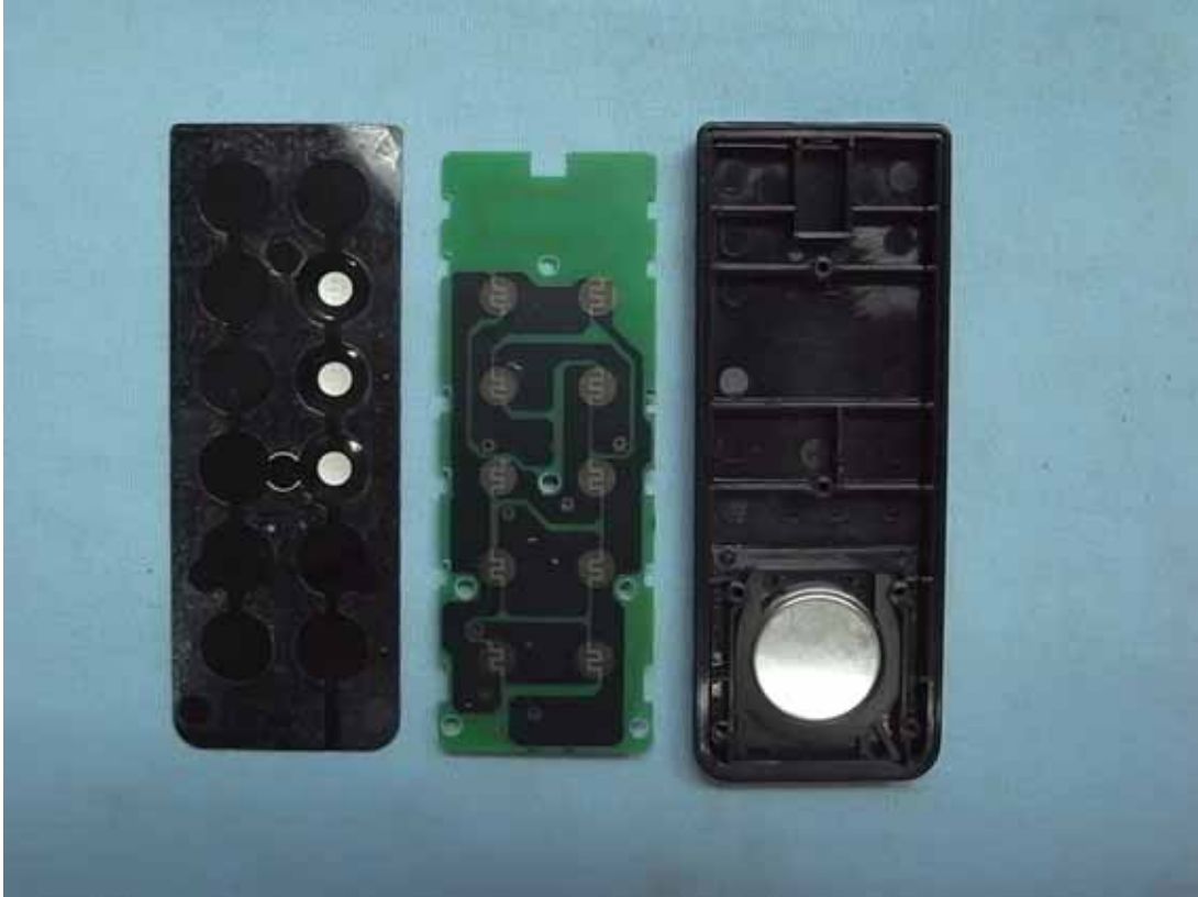
Figure 3 Internal View (Removed PCB)
