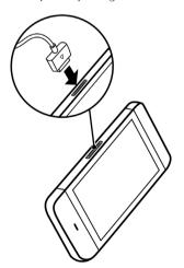
**NOTE:** The device is fully charged within four hours from a power outlet.
