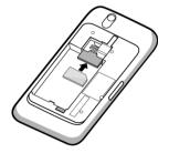
**NOTE:** If you have trouble inserting the card, ensure that you have aligned the angled corner on the card with the corner of the card holder.
