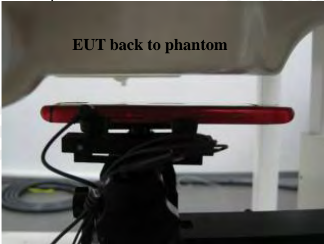
Fig.9 Body worn- EUT back to flat phantom and distance between flat phantom and mobile phone is 1.5 cm with headset
