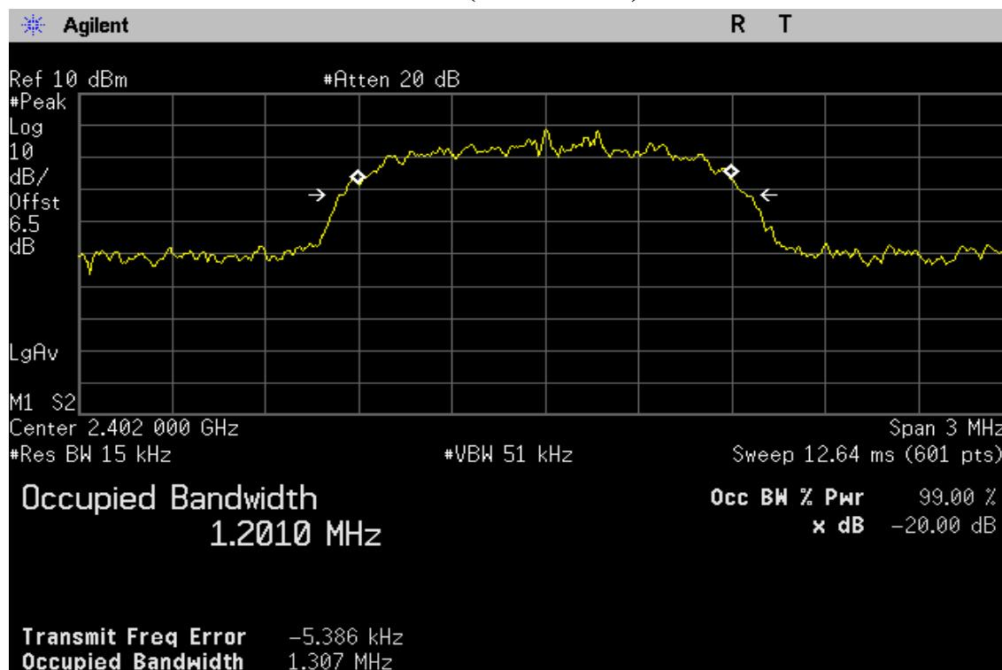
**20dB Band Width Test Data CH-Mid (EDR mode)**
