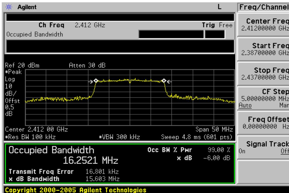
**6dB Band Width Test Data CH-Mid**
