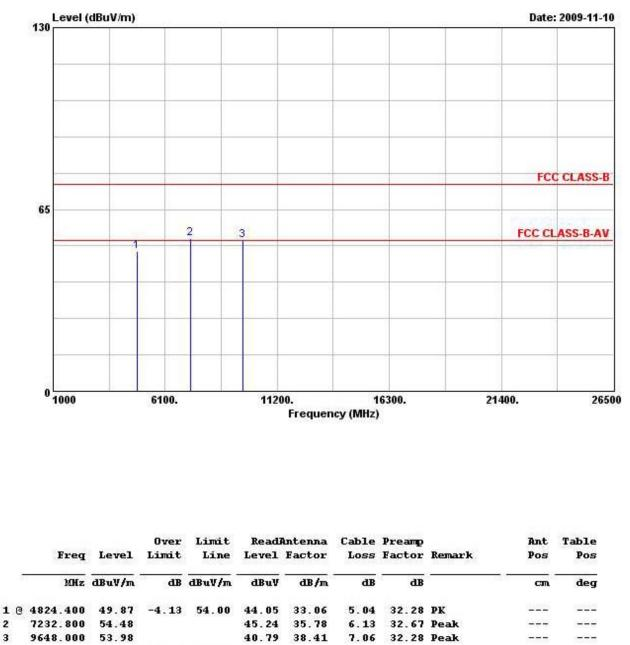
Note: An item 2 and 3 are on un-restricted band, so the limit is -20dB for the field strength of the fundamental emissions (see section 3.6.7).
