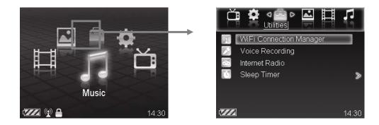
2. Select "Wi-Fi Connection Manager" and press the Navigation track ball to enter. The WLAN is off by default.
