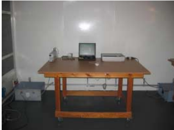
Photograph 9.1.1 Setup for conducted emission measurements
