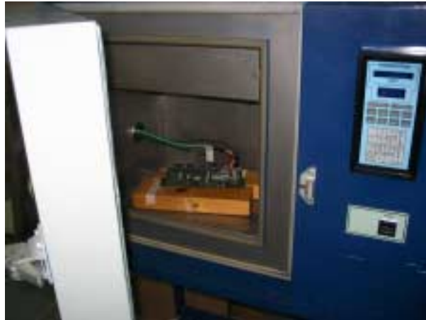
Photograph 7.5.1 Frequency stability test setup
