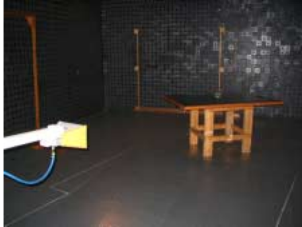
Photograph 9.2.2 Setup for radiated emission measurements, above 1 GHz
