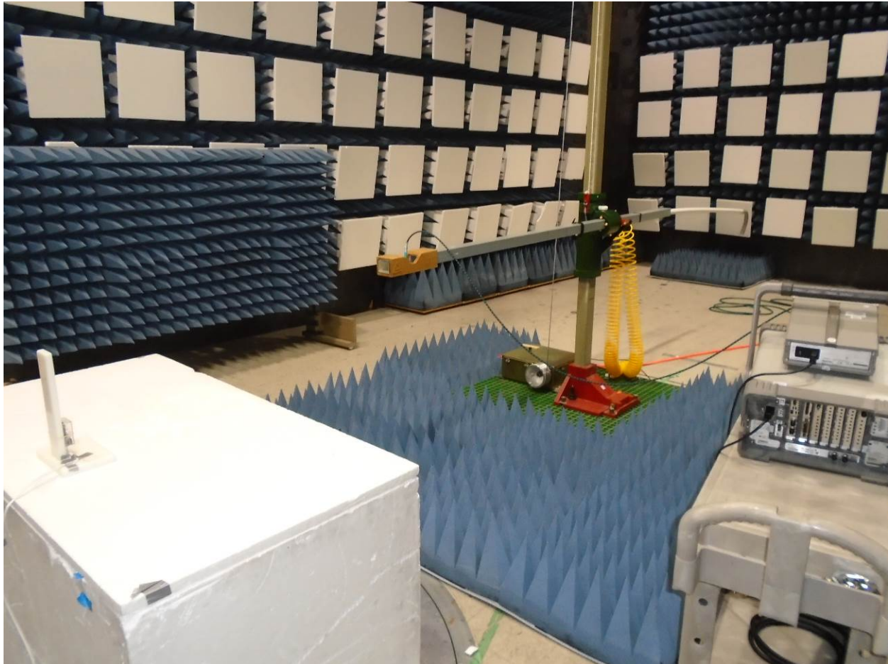
Figure 4: Typical Radiated Emissions – 18 GHz to 25 GHz shown, to ANSI C63.10:2009
