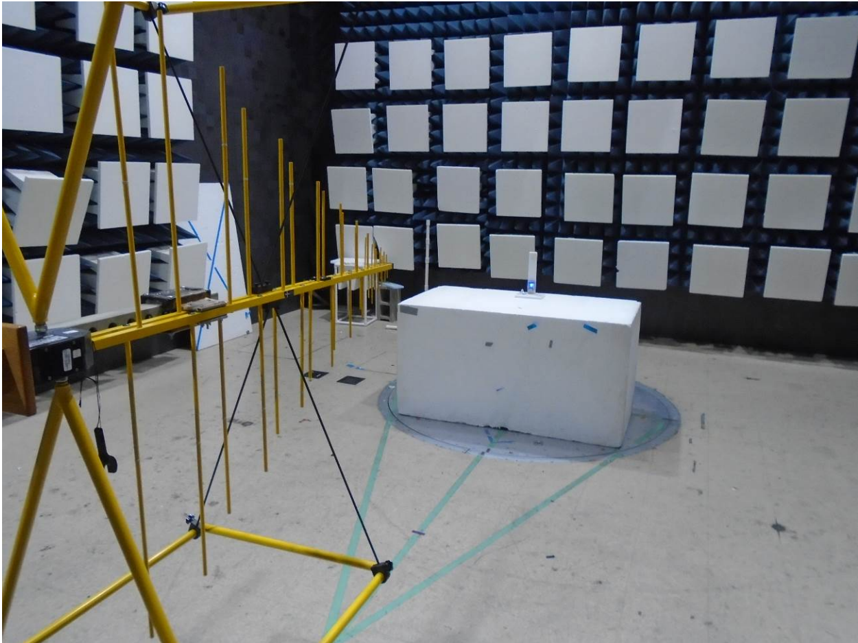
Figure 1: Typical Radiated Emissions – 30 MHz to 1 GHz shown, front view
