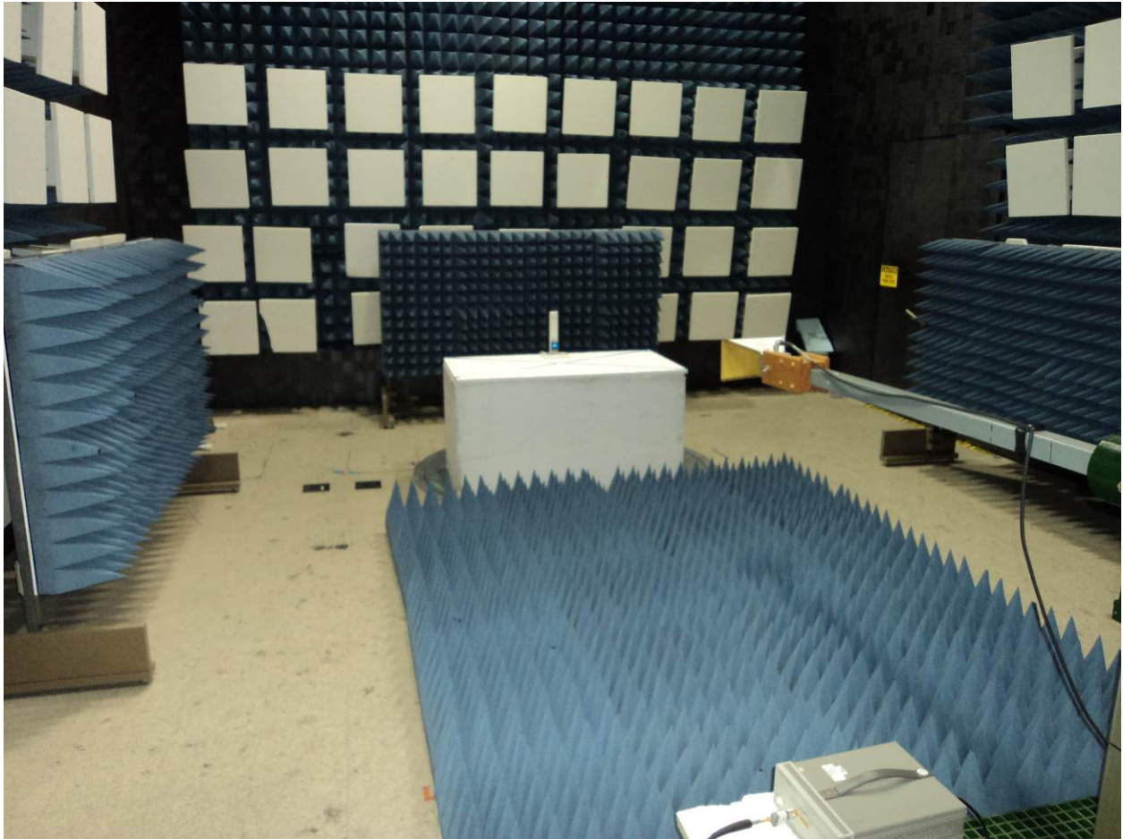
Figure 3: Typical Radiated Emissions – 1 GHz to 18 GHz shown, to ANSI C63.10:2009
