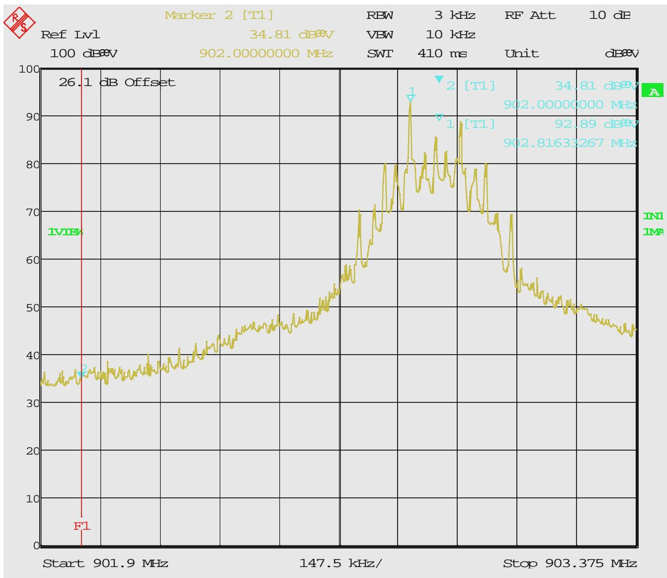
Notes: Measured using the Peak detector. Band Edge is at 902 MHz (Line F1 and Marker 2).
