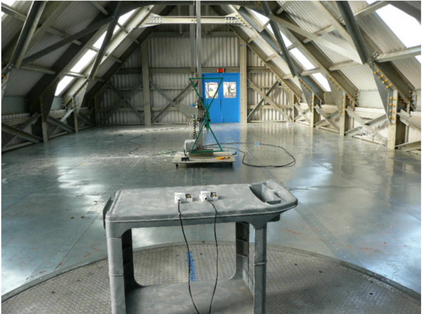
Figure 32 - Radiated Spurious Emissions Test Setup (Radiated Final Test - OATS)
