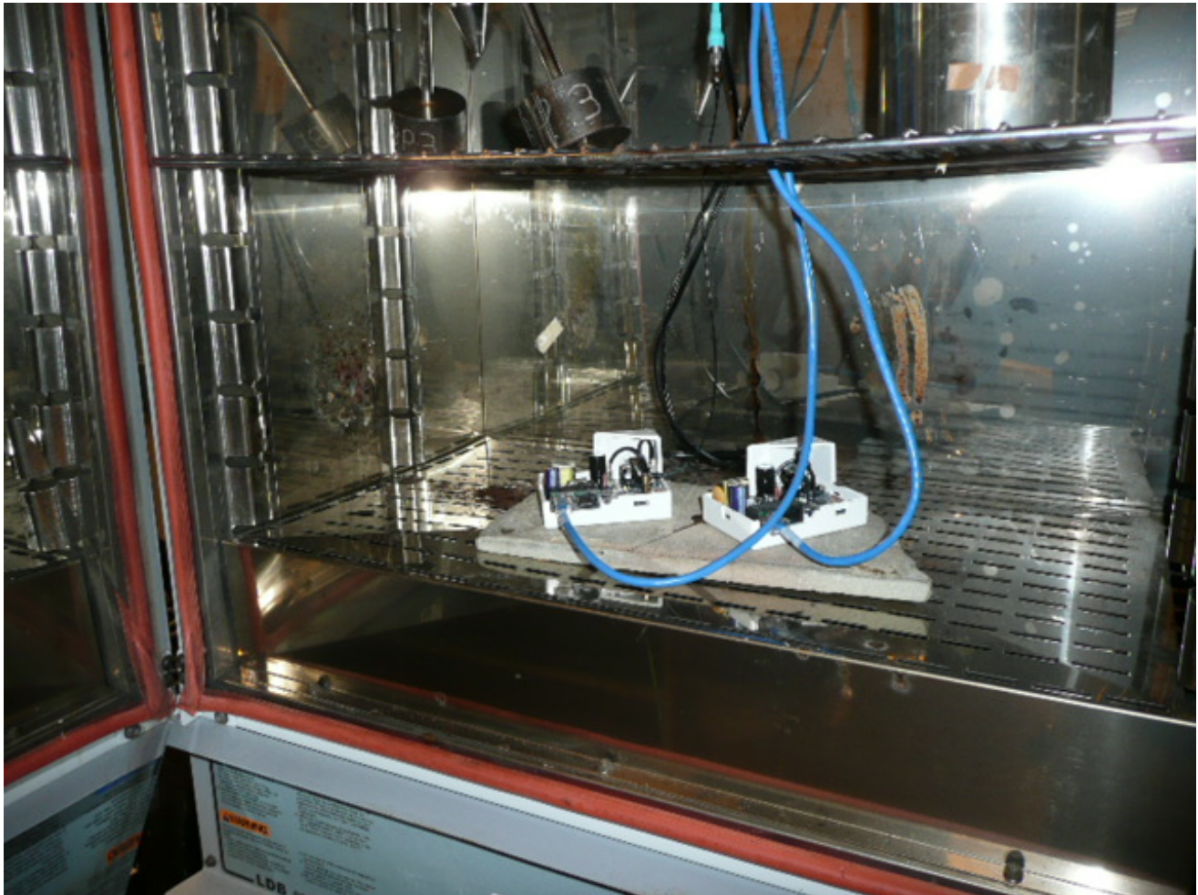
Figure 38 –Frequency Stability Test Setup – Temperature Chamber
