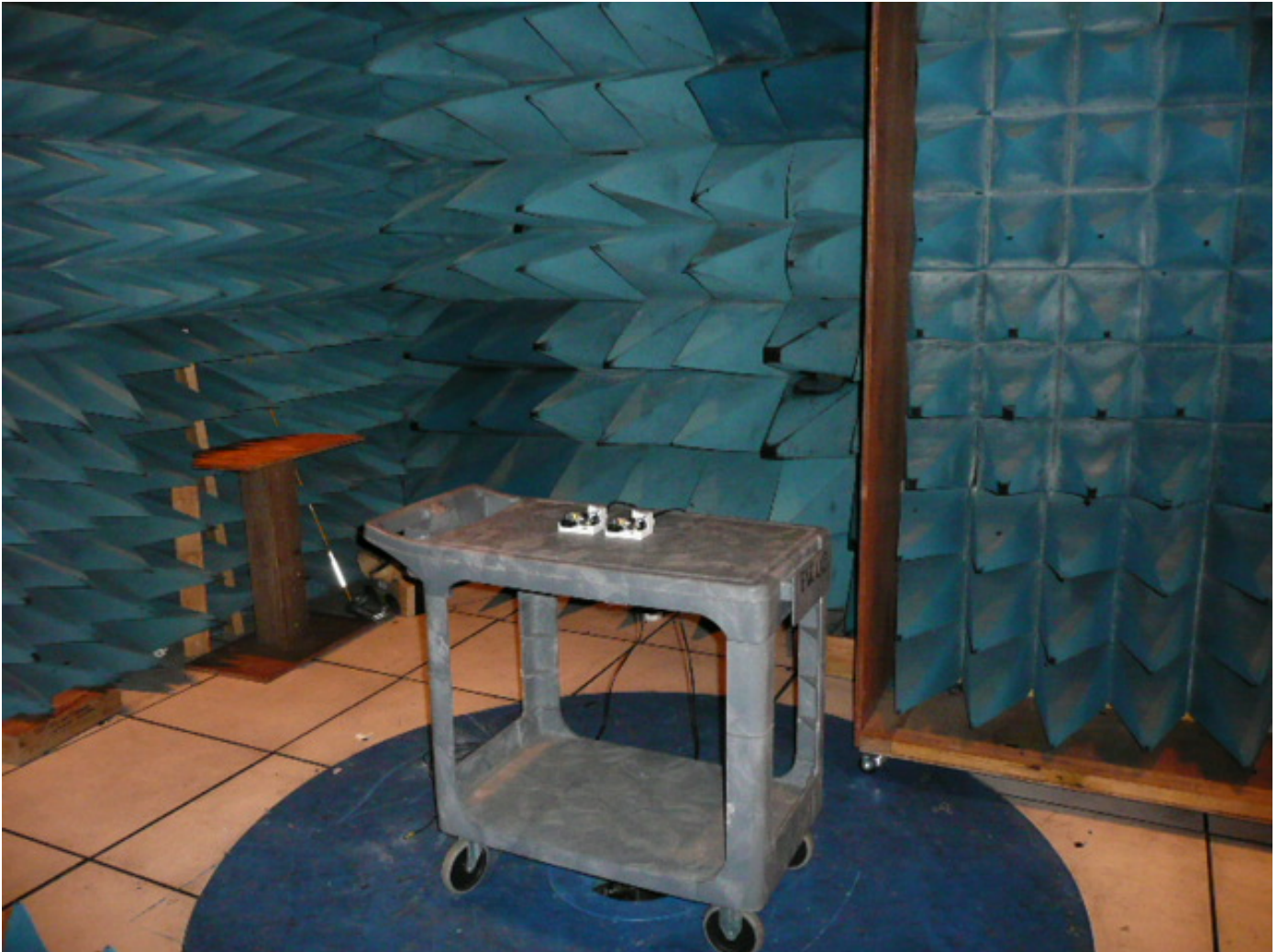
Figure 31 - Radiated Spurious Emissions Test Setup (Radiated Prescan- Semi Anechoic Chamber)
