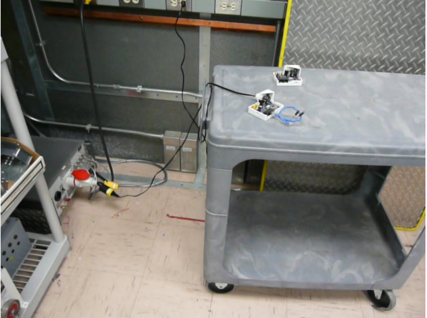
Figure 37 –Conducted Emissions Test Setup
