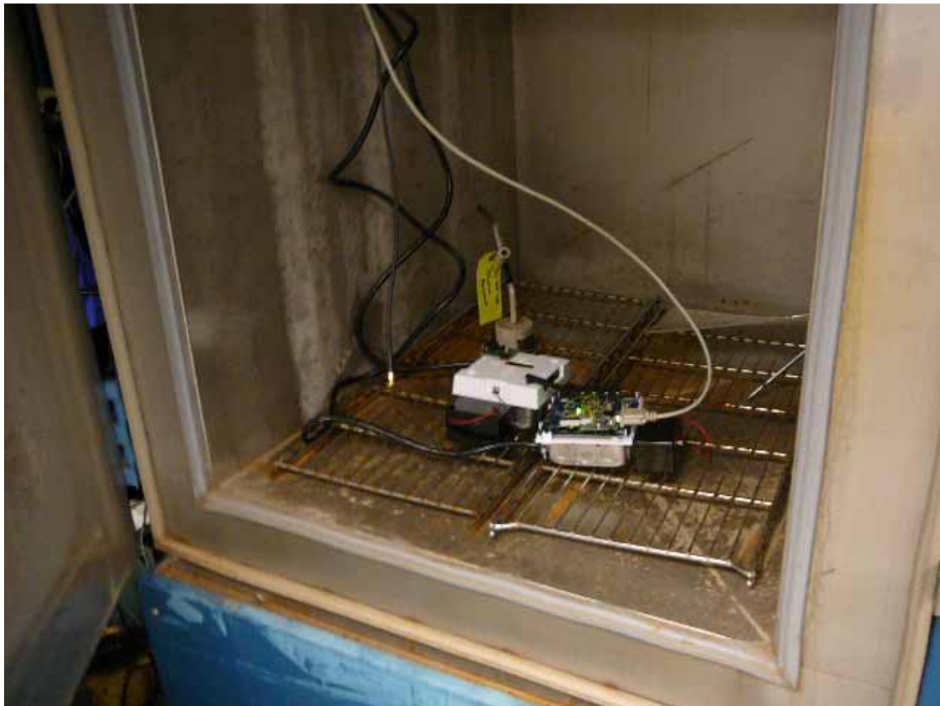
Figure 10 –Frequency Stability Test Setup – Humidity Chamber at 0°C
