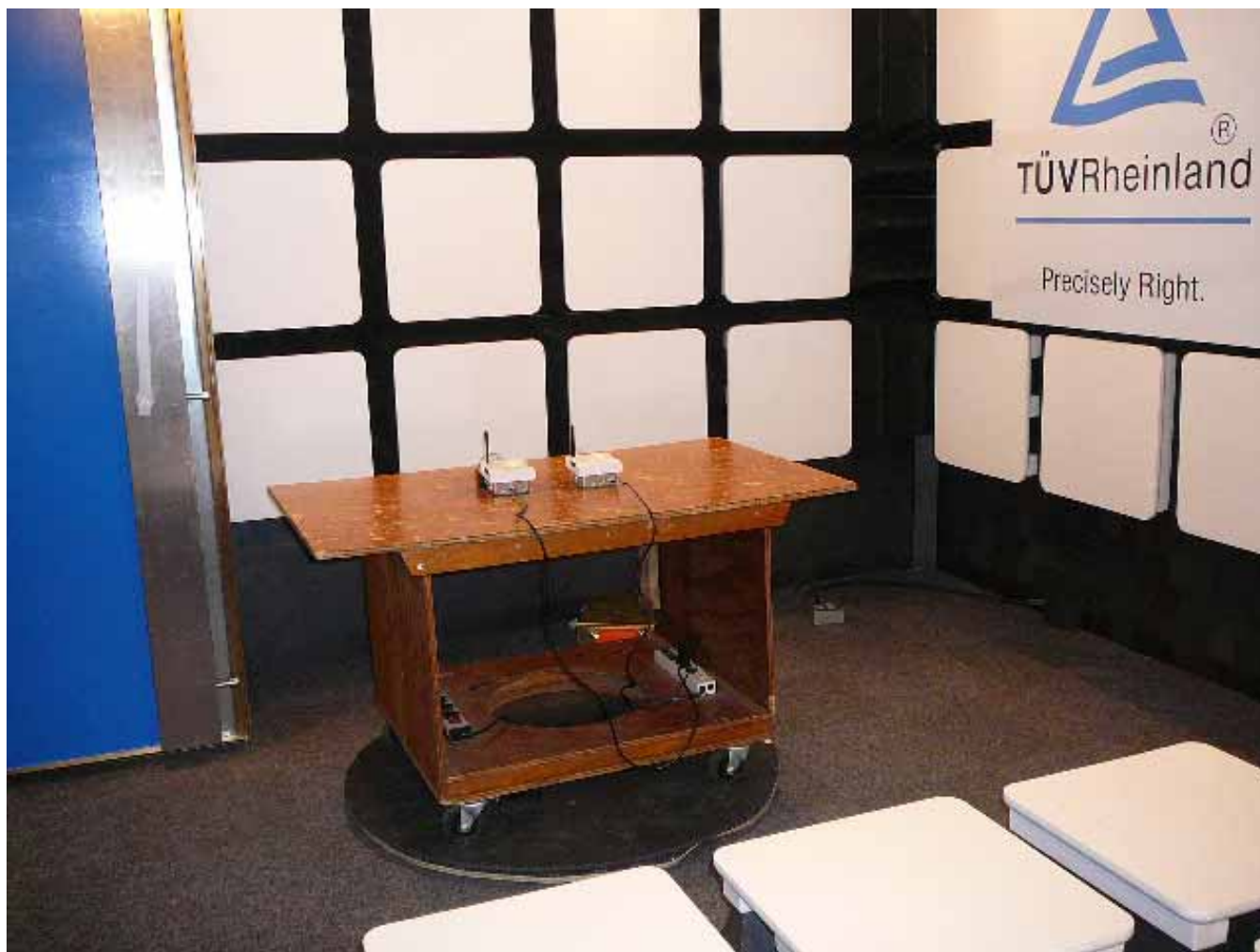
Figure 5 - Radiated Spurious Emissions Test Setup (Radiated Prescan- Semi Anechoic Chamber)
