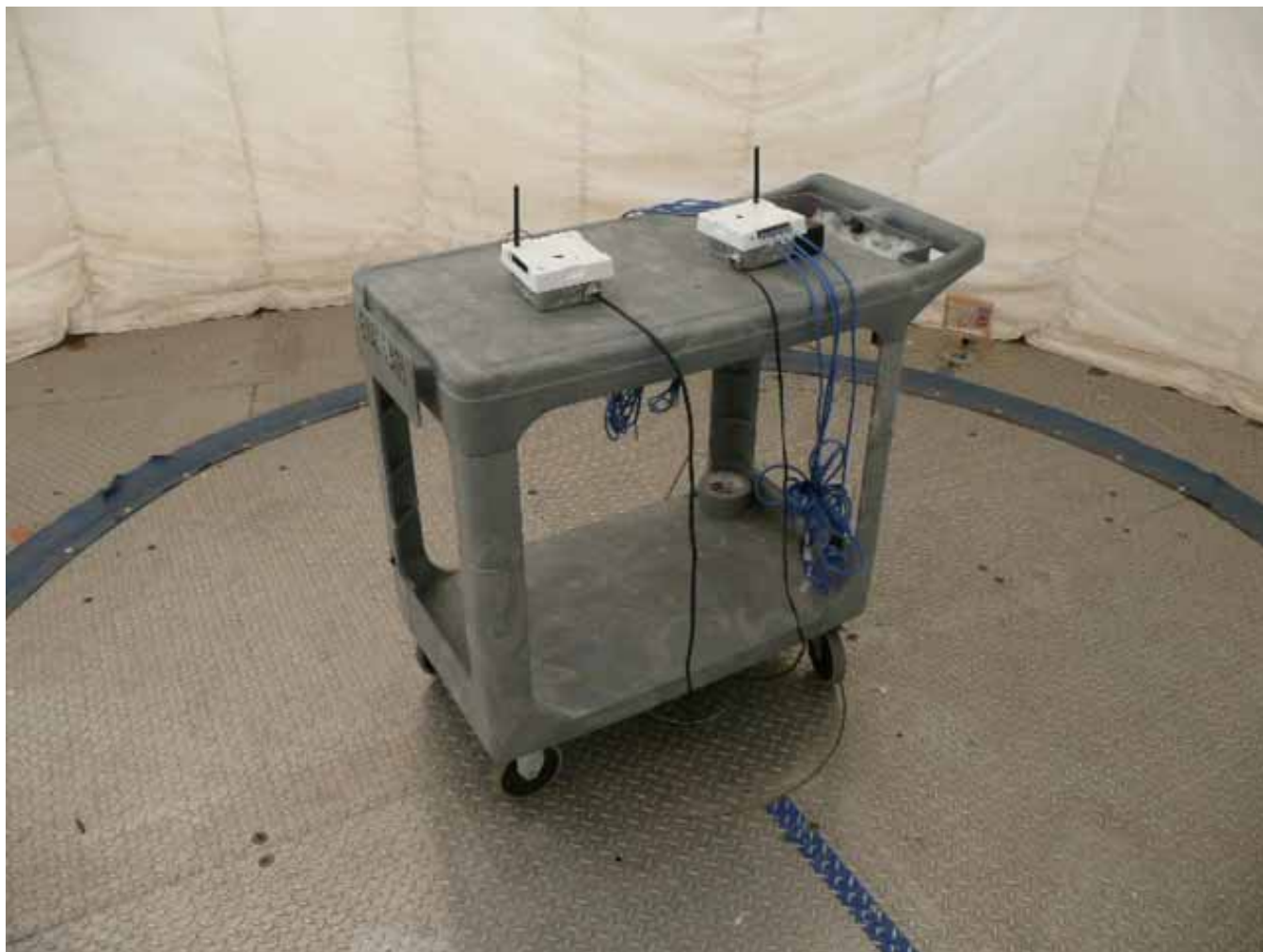
Figure 6 - Radiated Spurious Emissions Test Setup (Radiated Final Test - OATS)
