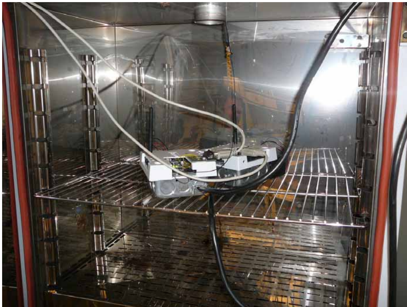
Figure 9 –Frequency Stability Test Setup – Temperature Chamber at +50°C
