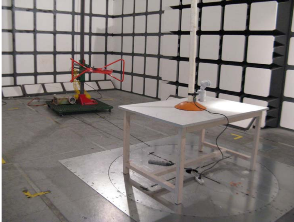
Radiated Emission - Front View (Below 1GHz)
