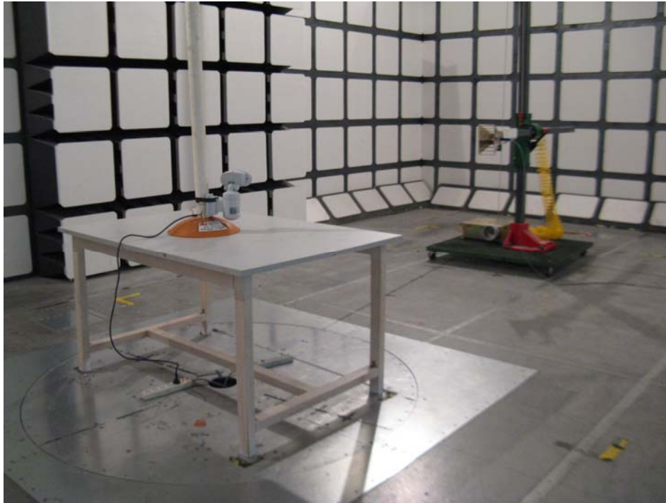
Radiated Emission - Rear View (Above 1GHz)
