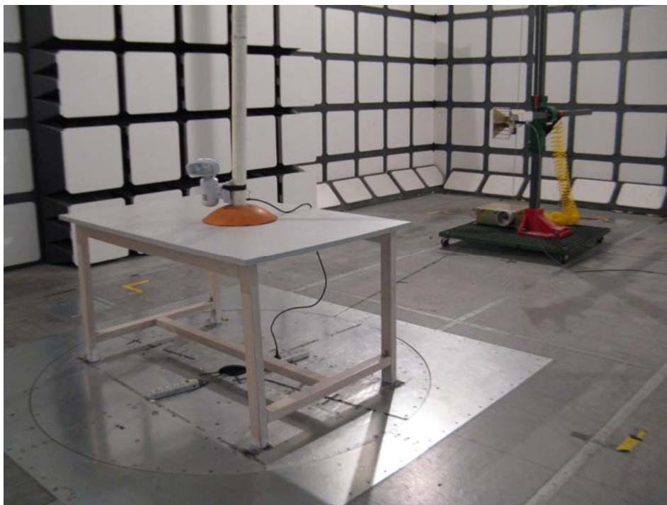
Radiated Emission - Rear View (Above 1GHz)
