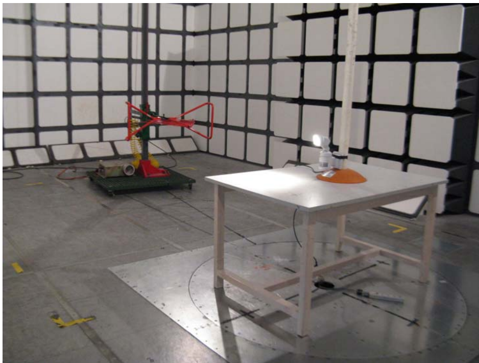
Radiated Emission - Rear View (Below 1GHz)
