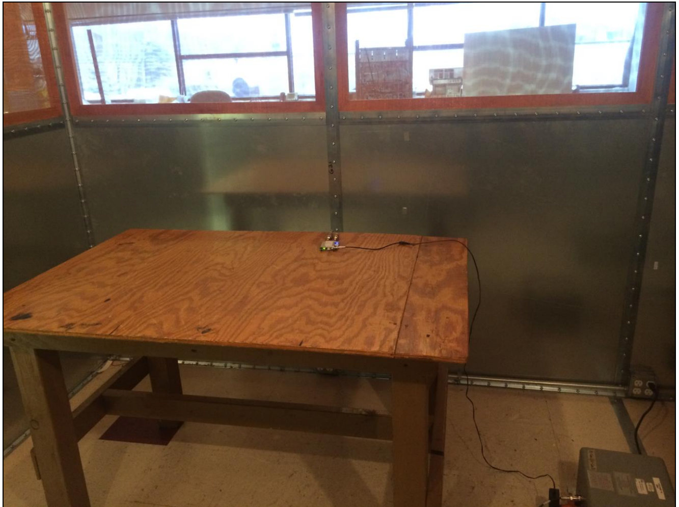
Photograph 2. Conducted Emissions, Test Setup
