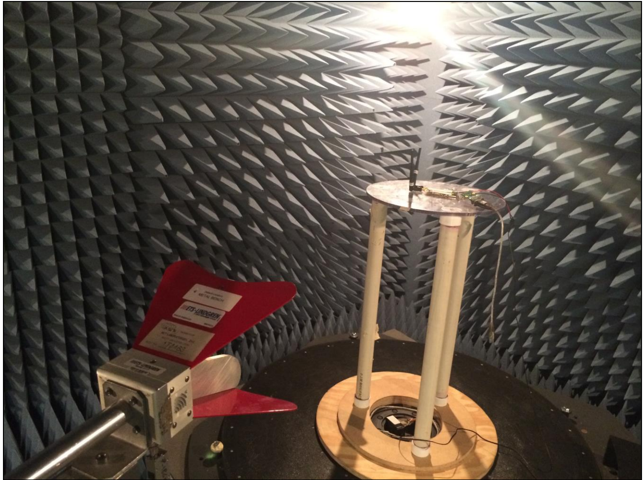
Photograph 5. Radiated Spurious Emissions, Test Setup Above 1 GHz
