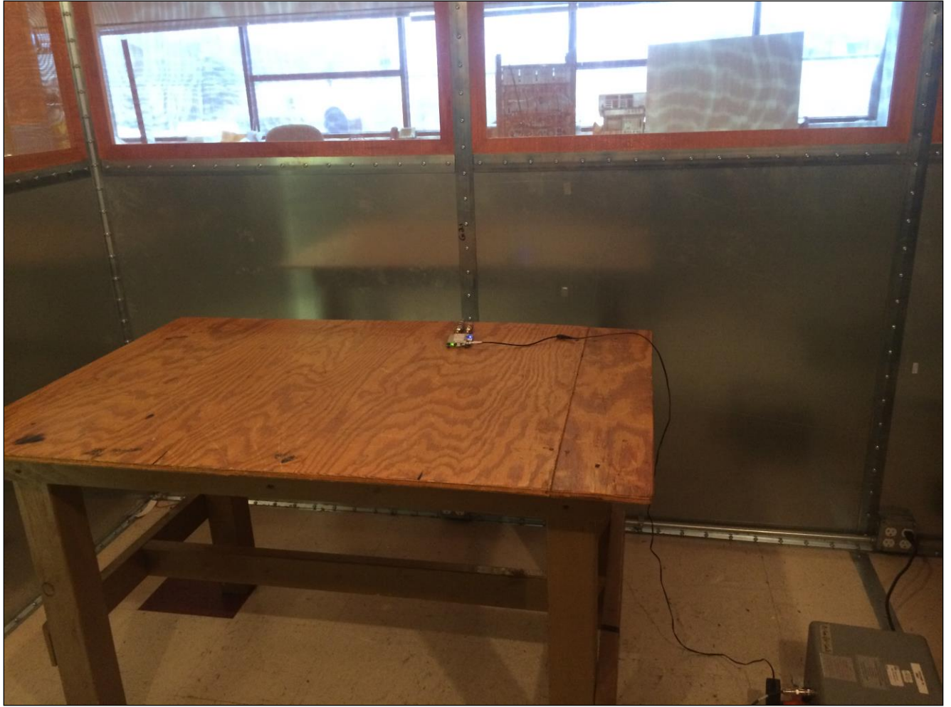
Photograph 1. Conducted Emissions, Test Setup
