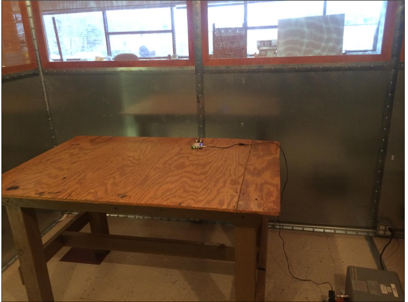
Photograph 3. Conducted Emissions, §15.207, Test Setup
