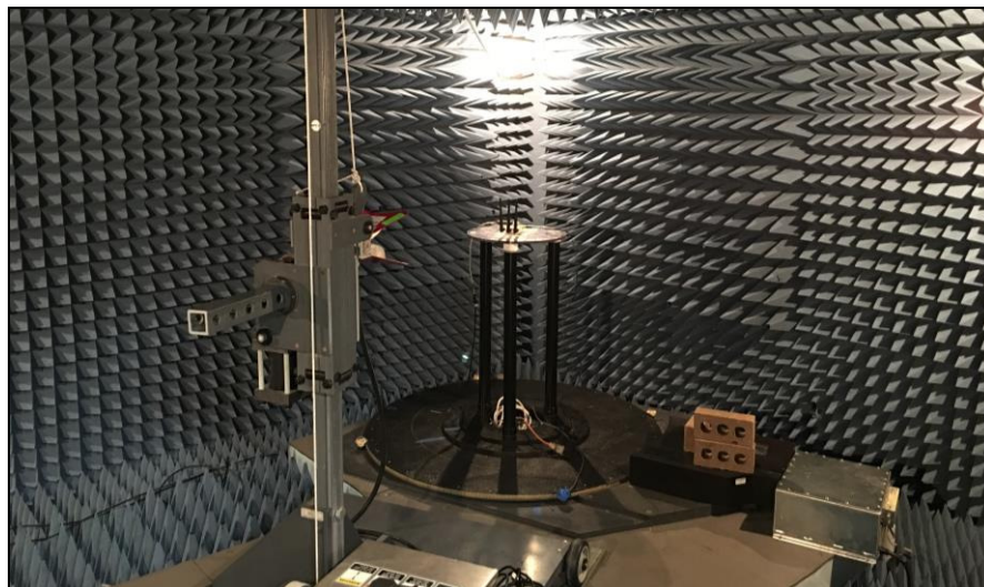
Photograph 2. Radiated Emissions, Test Setup Above 1GHz
