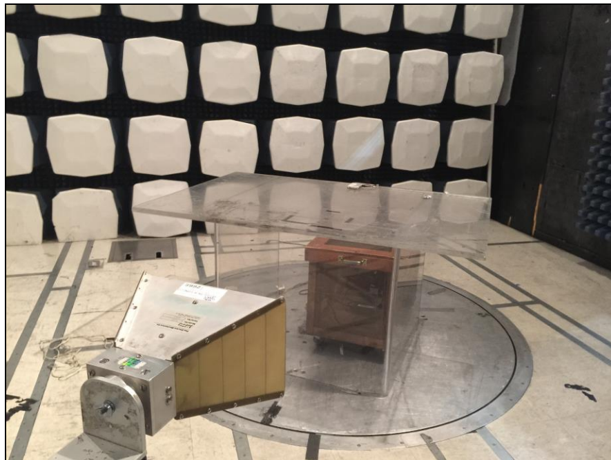
Photograph 2. Radiated Spurious Emissions, Test Setup, Above 1 GHz
