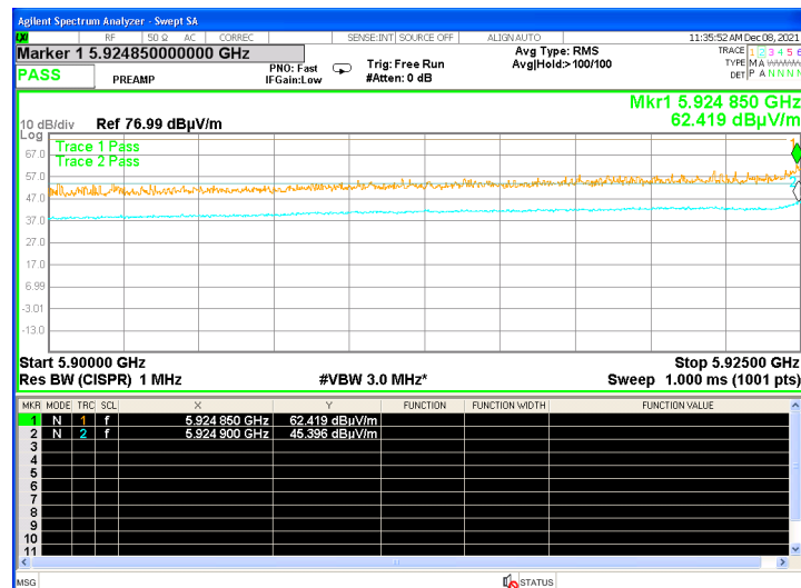
Figure 44 Fundamental: 5.945 GHz ,40 MHz, band 2
