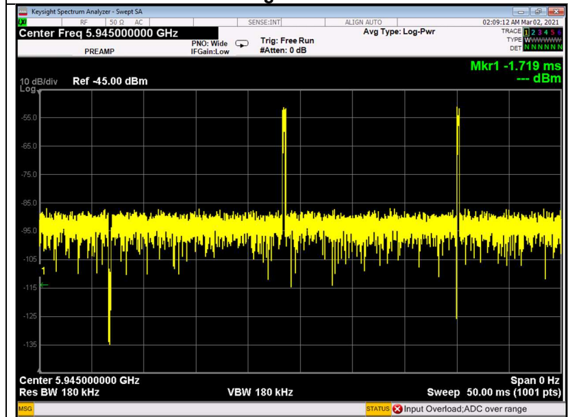
Figure 87. E.U.T transmission 5945.0MHz (40MHz BW) incumbent signal 5960.0MHz OFF
