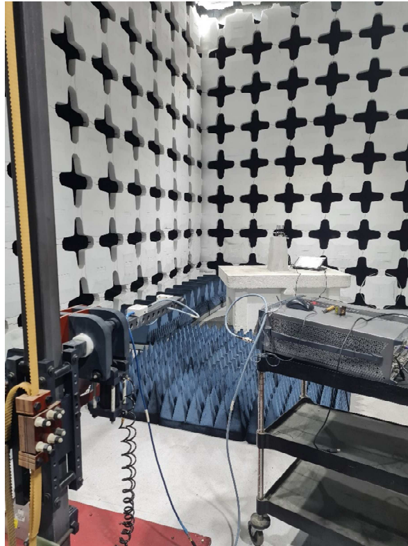
Figure 12. Radiated Emission Test, 15-40GHz
