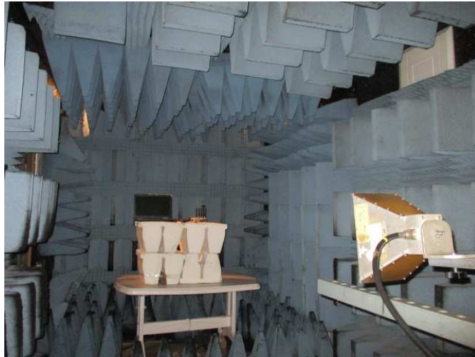
Figure 8. Band Edge screening setup, "mushroom" antenna
