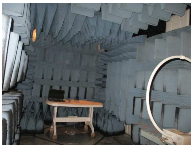
Figure 5. Radiated Emission Test, 0.009-30.0MHz
