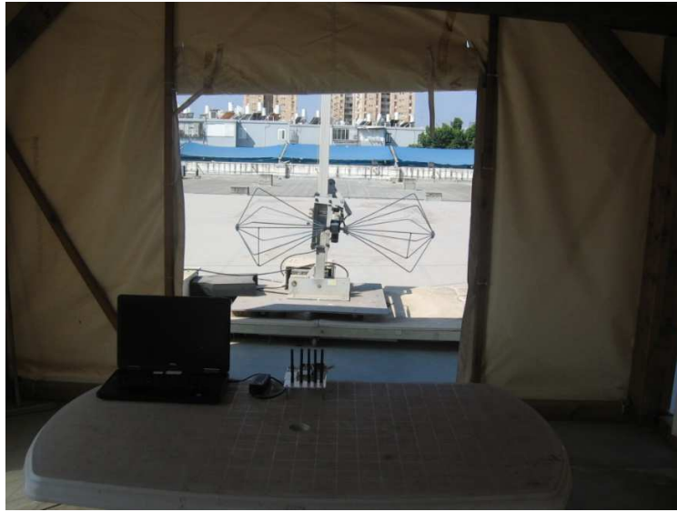
Figure 6. Radiated Emission Test, 30.0-200.0MHz
