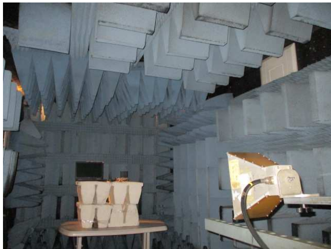
Figure 9. Band Edge screening setup, "dipole" antenna
