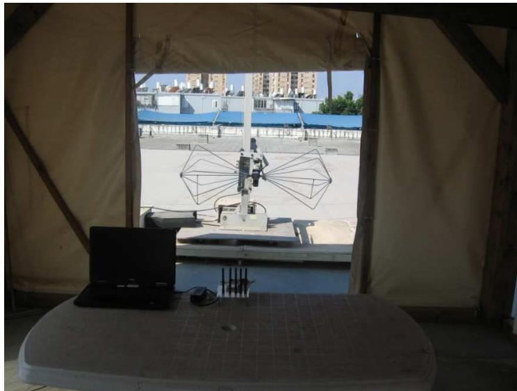
Figure 4. Radiated Emission Test, 30.0-200.0MHz
