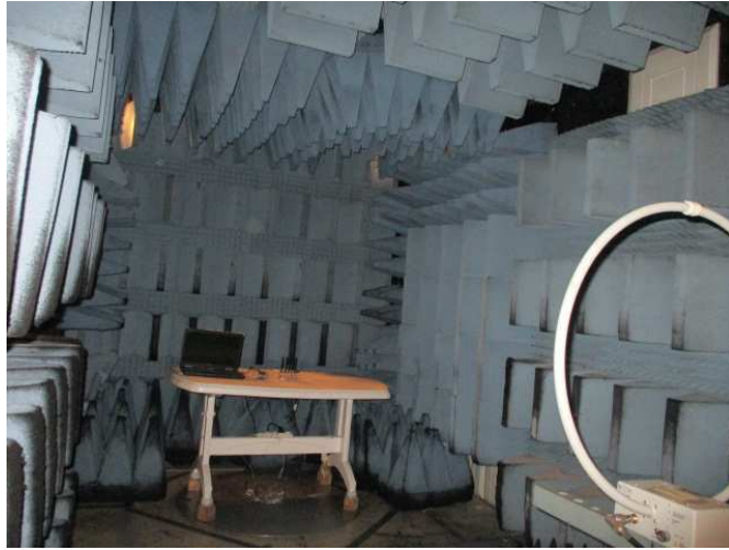
Figure 3. Radiated Emission Test, 0.009 30.0MHz
