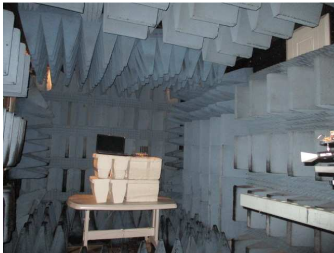
Figure 8. Radiated Emission Test, 26.5-40.0GHz
