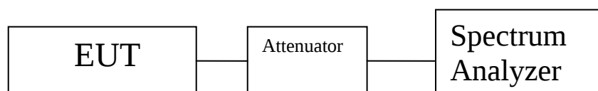
Figure 3. Occupied Bandwidth, Test Block Diagram
