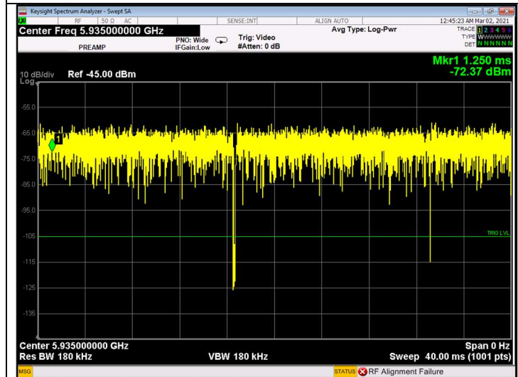
Figure 164. E.U.T transmission 5935.0MHz (20MHz BW) incumbent signal 5930.0MHz OFF
