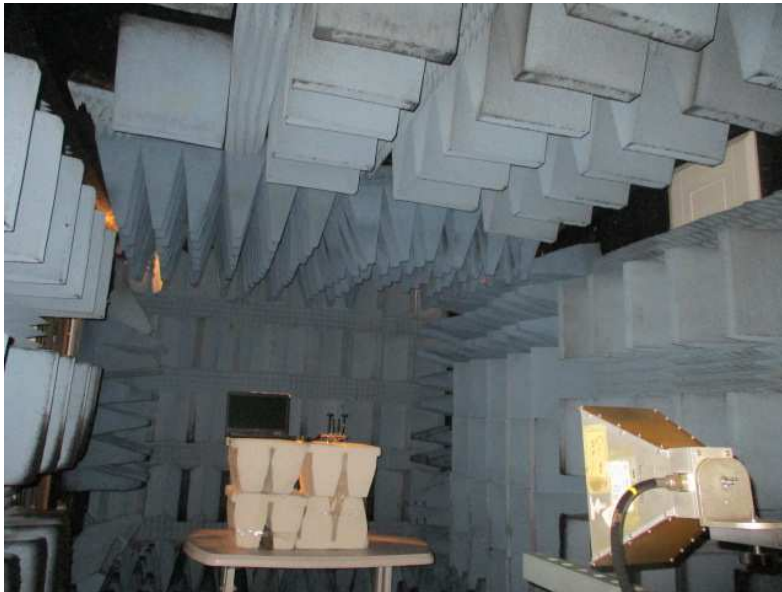
Figure 8. Band Edge screening set up, "mushroom" antenna
