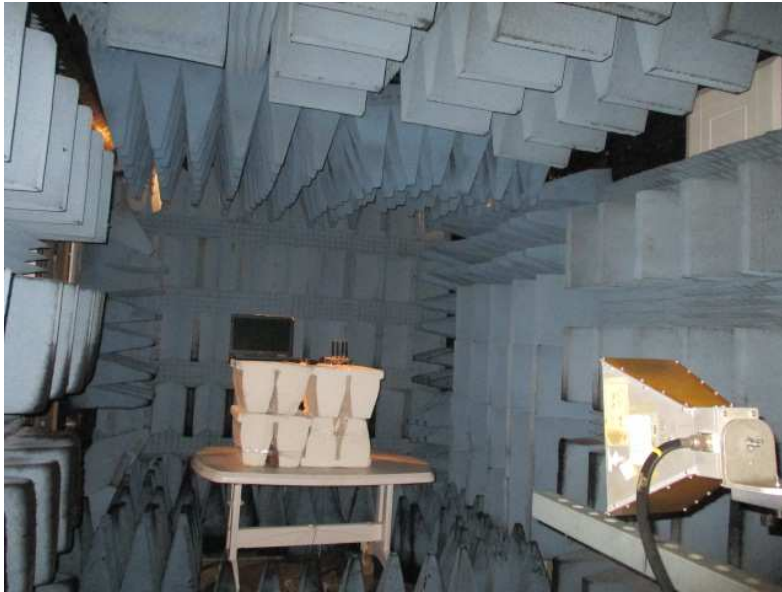
Figure 9. Band Edge screening set up, "dipole" antenna
