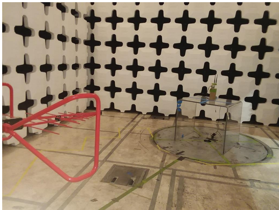
Photograph 4. Radiated Emissions, 2x2 Test Setup Below 1GHz
