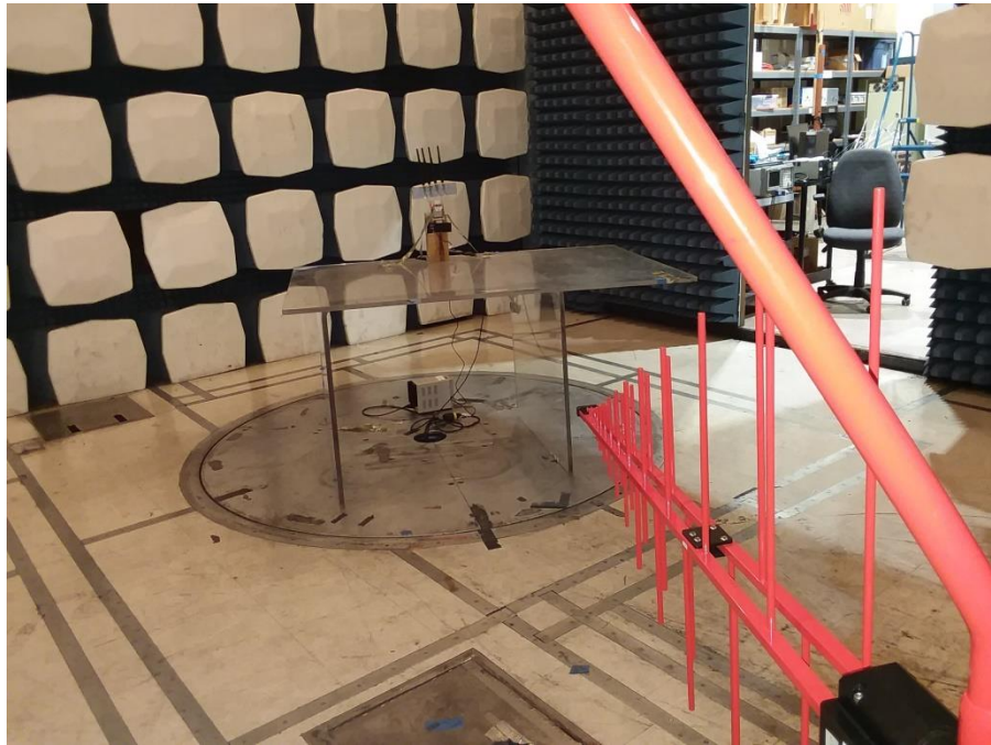
Photograph 1. Radiated Emissions, 4x4 Test Setup Below 1GHz
