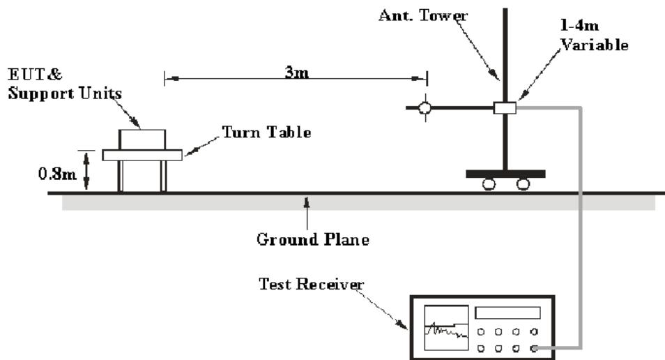
The radiated emission tests were performed in the 3 meters, using the setup accordance with the ANSI C63.4-2009. The specification used was the FCC 15.209, and FCC 15.407 limits.
