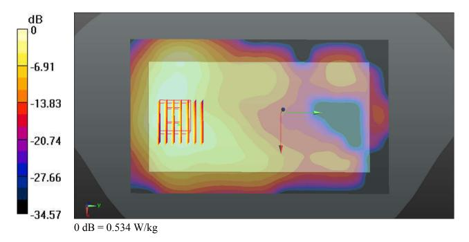
Communication System: UID 0, WIFI (0); Frequency: 2412 MHz; Duty Cycle: 1:1
