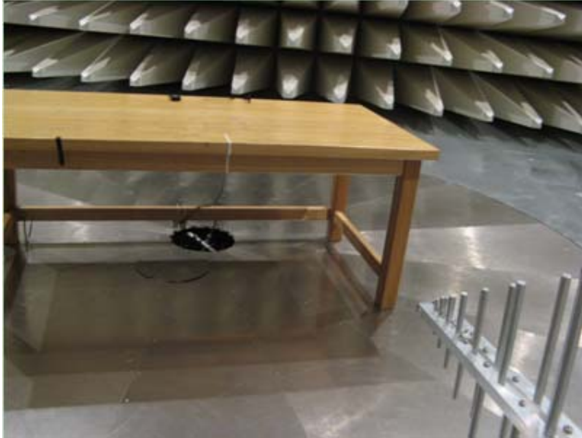
Photo of Radiated Emission Test
