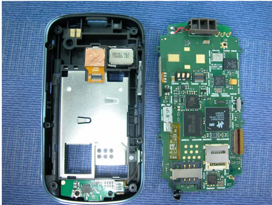
Mobile phone Disassembly
