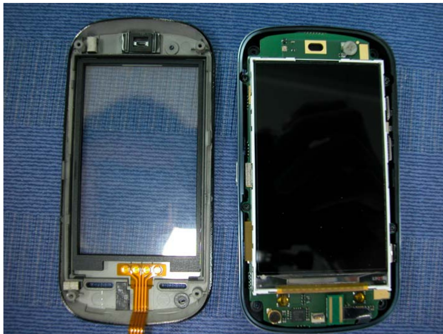
Mobile phone Disassembly
