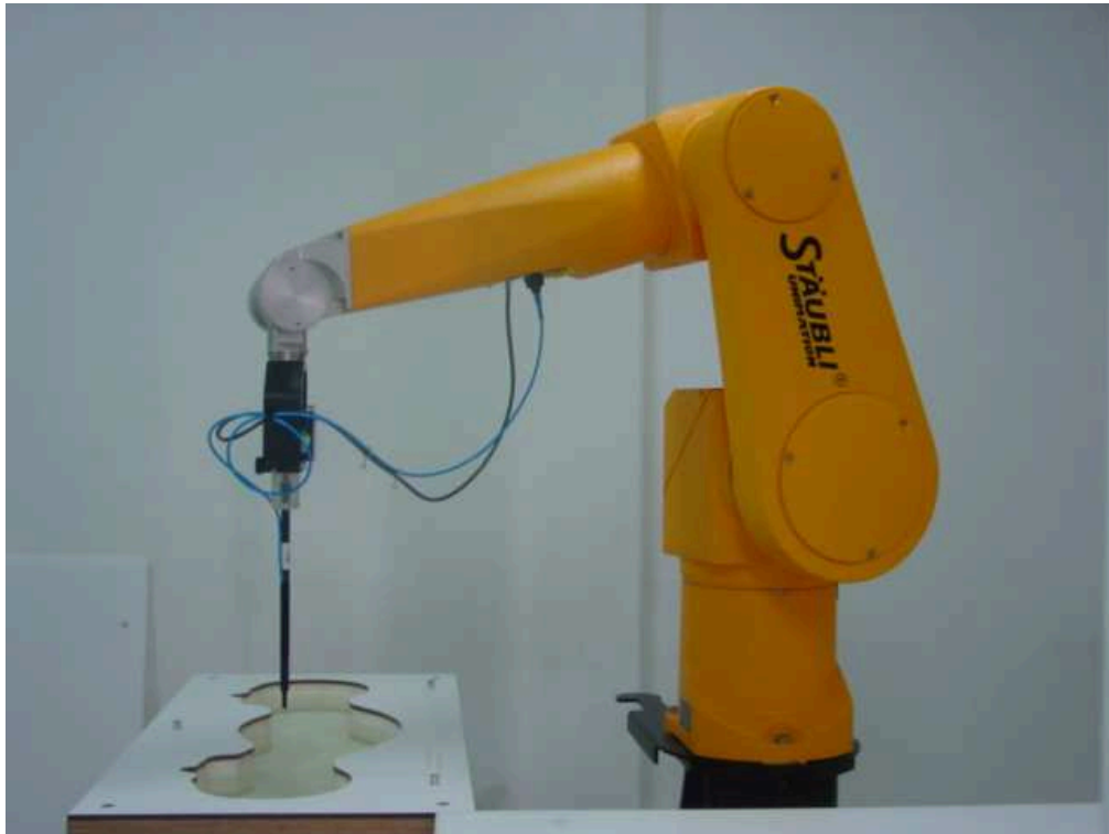
Picture B1: Specific Absorption Rate Test Layout
