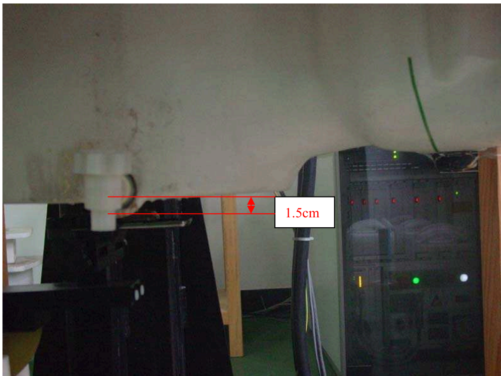
Picture B10: Body-worn Position with Bluetooth transmitter on (towards ground, the distance from handset to the bottom of the Phantom is 1.5cm)
