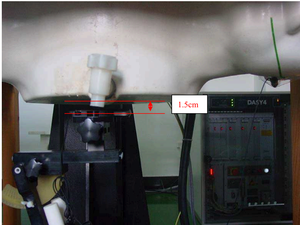
Picture B9: Body-worn Position with a headset (towards ground, the distance from handset to the bottom of the Phantom is 1.5cm)
