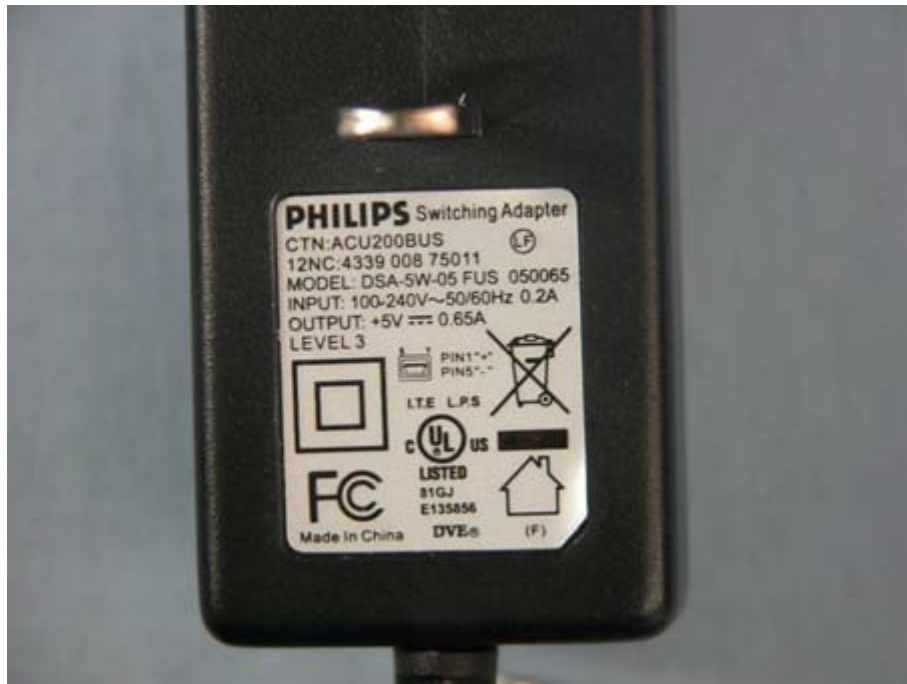
Label of Charger (AC/DC Adapter)
