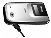
The battery symbol indicates the state of charge. During charging, the charge indicators will scroll; it takes around 4 hours to fully charge the battery. When all the scroll bars are steady, the battery is fully charged. You can then disconnect the charger. Depending on the network and condition of use, talk time and stand-by time can go up to 16 hours\* and 1440 hours (2 months)\* respectively.
