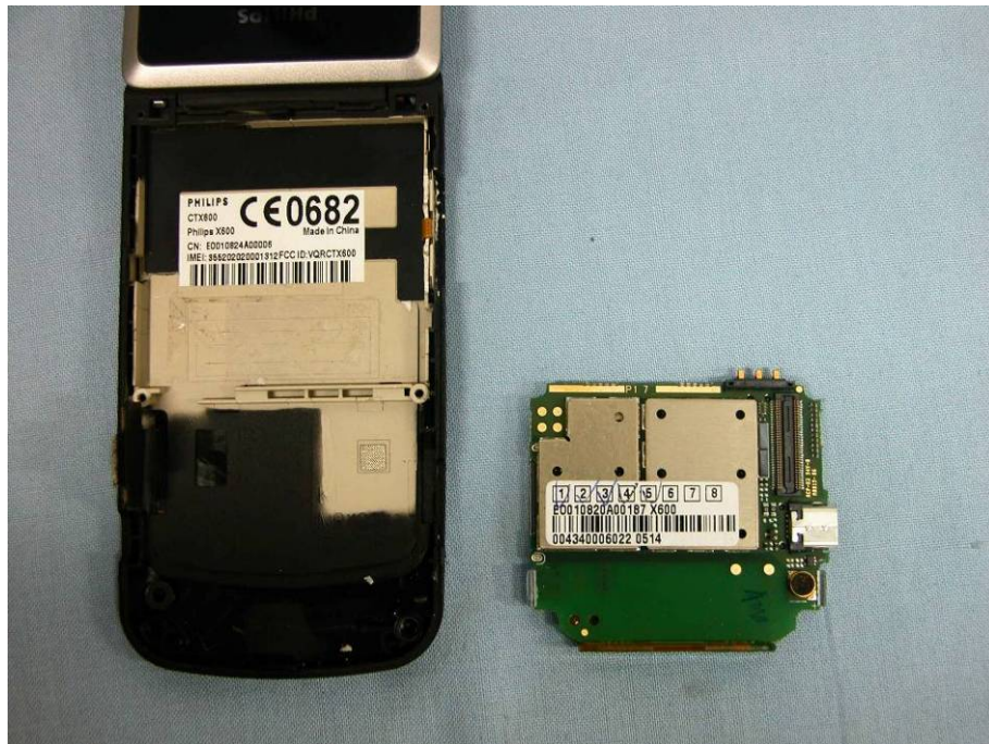
Mobile phone Disassembly
