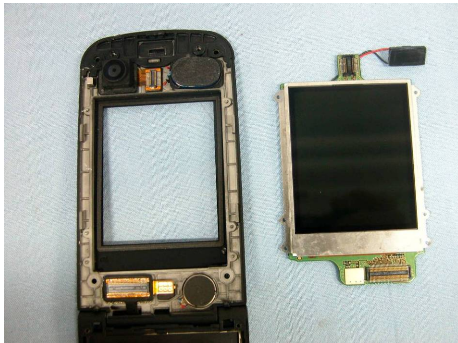
Mobile phone Disassembly
