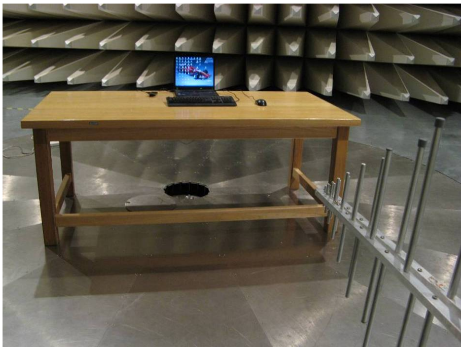
Pic C-2 Radiated Spurious Emission
