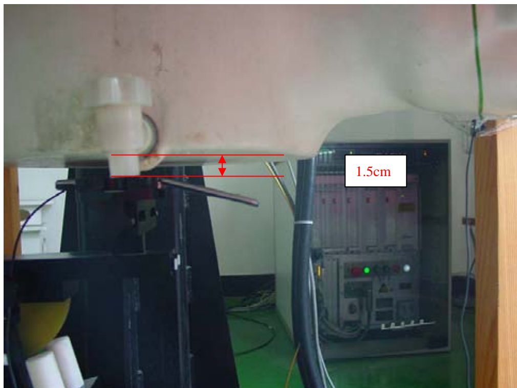
Picture B8: Body-worn Position with headset (towards ground, the distance from handset to the bottom of the Phantom is 1.5cm)
