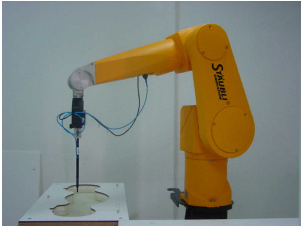
Picture B1: Specific Absorption Rate Test Layout
