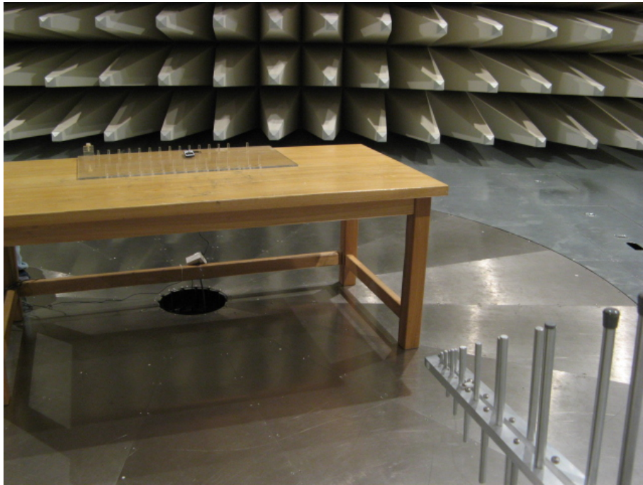
Pic C-3 Radiated Spurious Emission (Charging Mode)
