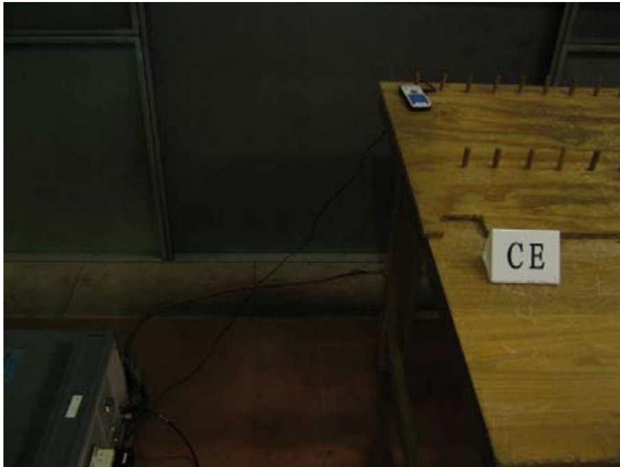
Pic C-1 Conducted Emission (Charging Mode)
