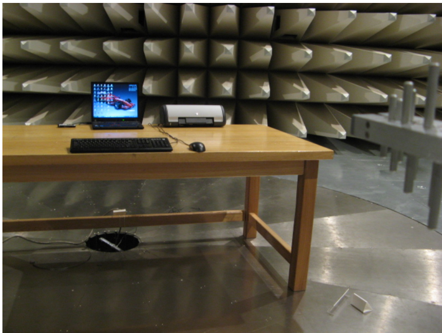
Pic C-4 Radiated Spurious Emission (USB Mode)
