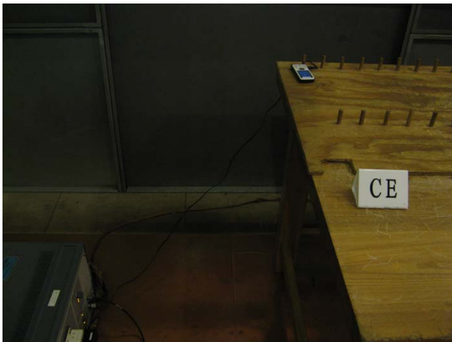
Photo of AC Powerline Conducted Emission Test
