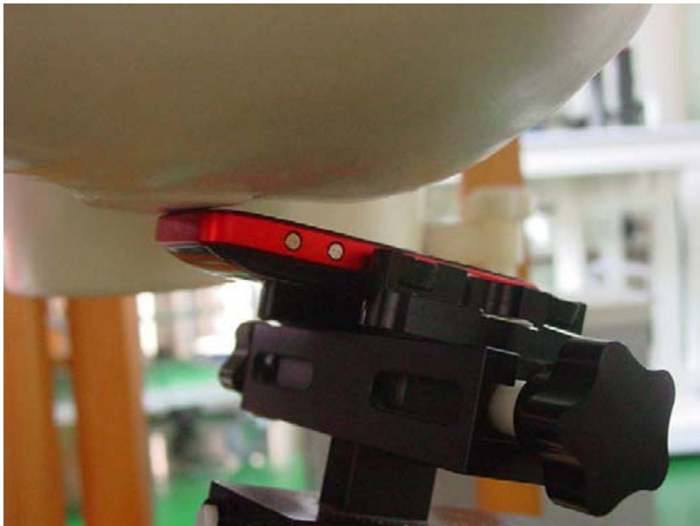
Picture B7: Right Hand Tilt 15° Position
