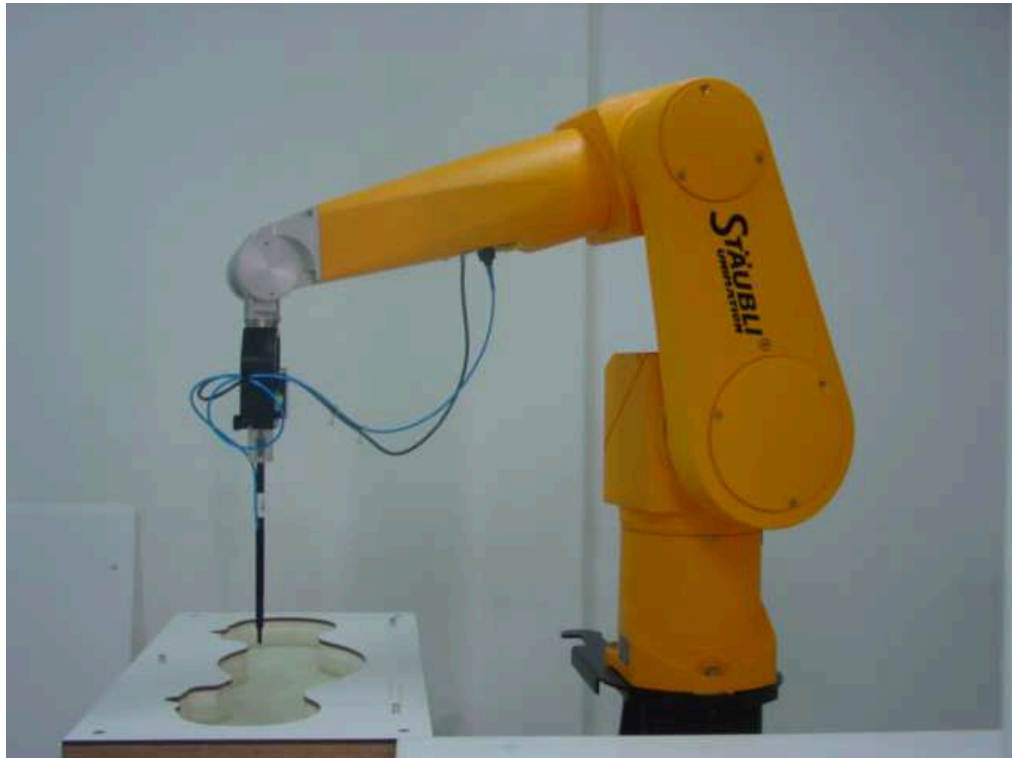
Picture B1: Specific Absorption Rate Test Layout
