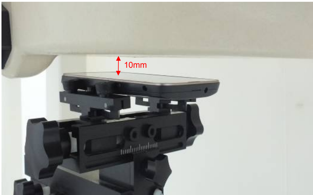
Picture 14: Front Side, the distance from handset to the bottom of the Phantom is 10mm
