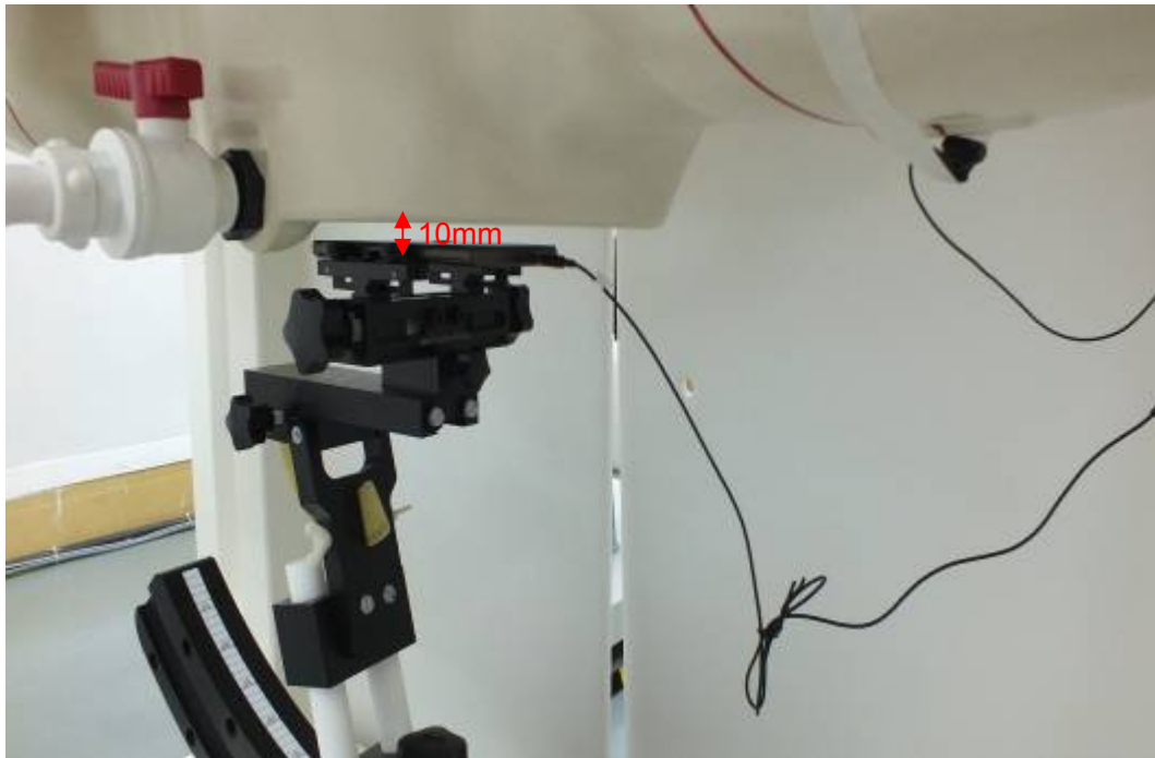
Picture 19: Back Side with earphone, the distance from handset to the bottom of the Phantom is 10mm
