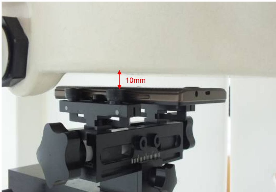
Picture 13: Back Side, the distance from handset to the bottom of the Phantom is 10mm
