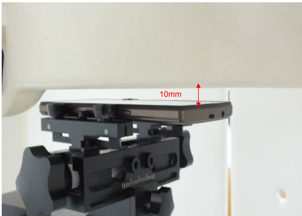
Picture 14: Front Side, the distance from handset to the bottom of the Phantom is 10mm
