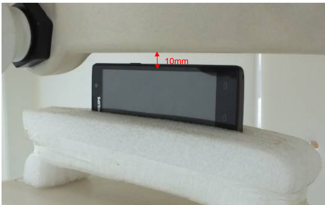
Picture 16: Right Edge, the distance from handset to the bottom of the Phantom is 10mm
