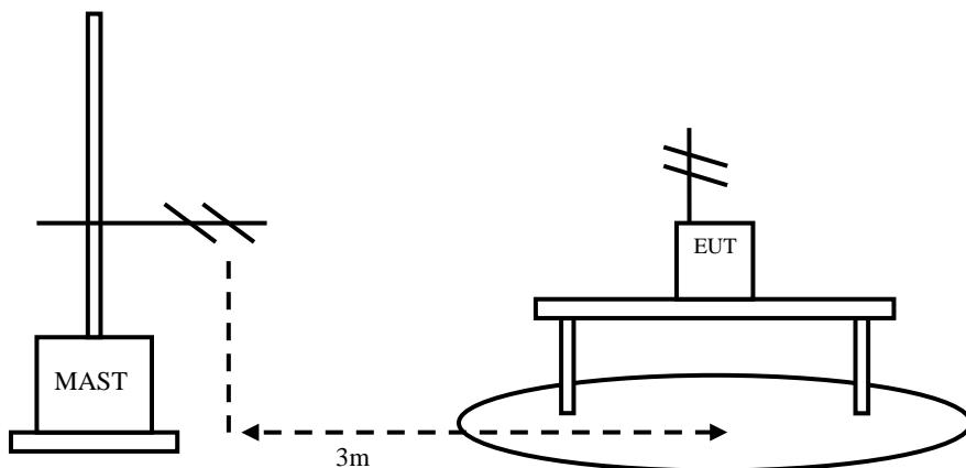
The Equipment Under Test (EUT) was set up on a non-conductive table in the semi-anechoic chamber. The test was performed at the distance of 3 m between the EUT and the receiving antenna. The radiated emissions measurements were made in a typical installation configuration. Then start the test software ES-K1. Sweep the whole frequency band through the range from 30MHz to 1GHz or above, using receive log period antenna HL562 or Ridge horn antenna HF906.
