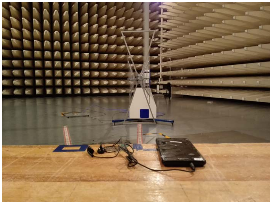
Spurious Radiated Emissions Test setup (30MHz~1GHz)
