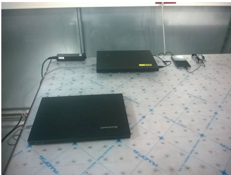
Conducted Emissions Test Setup (with laptop)
