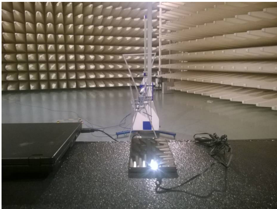
Radiated Emissions Test Setup (with laptop)
