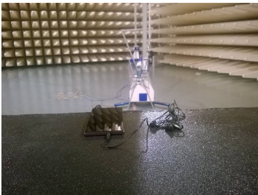
Radiated Emissions Test Setup (with charger)
