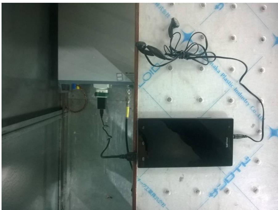
Conducted Emissions Test Setup (with charger)
