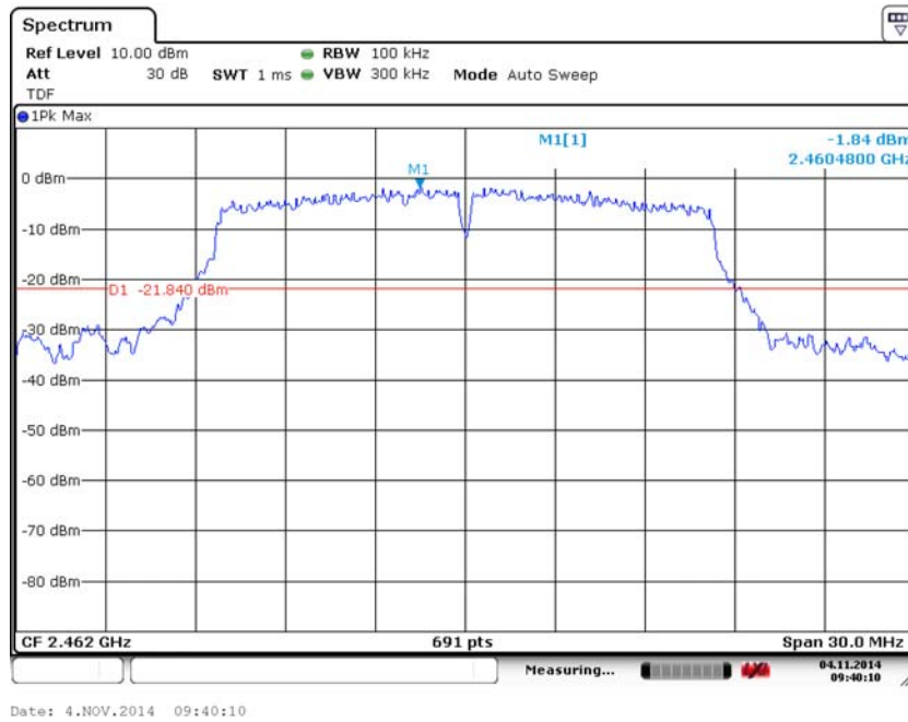
Fig. 132 Conducted Spurious Emission (802.11g, Ch11, Center Frequency)
