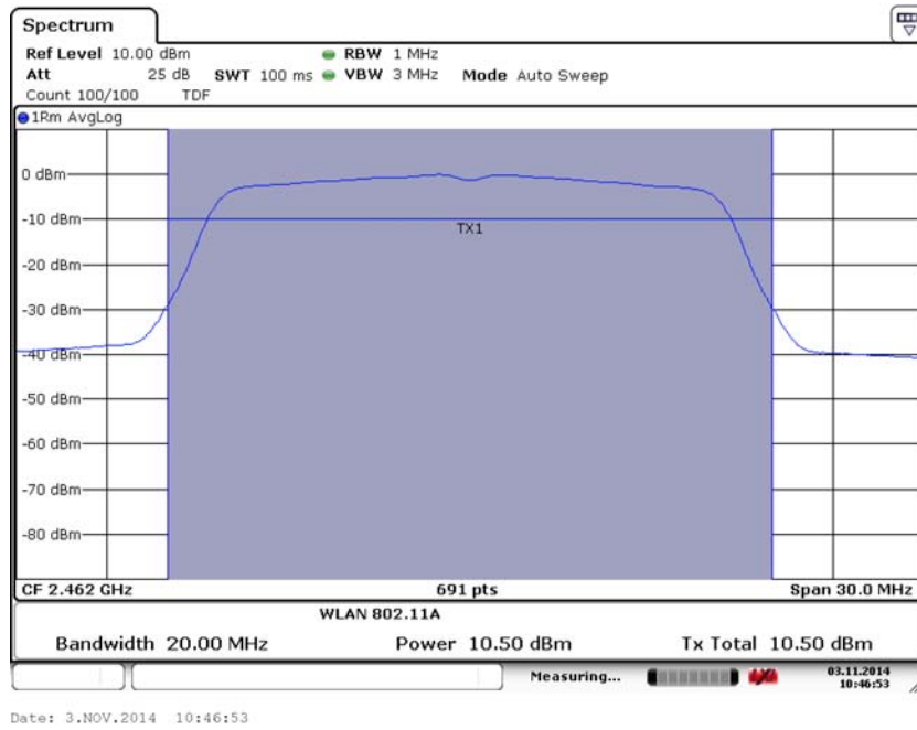
Fig. 15 Maximum Average Output Power (802.11g, Ch 11,6Mbps)
