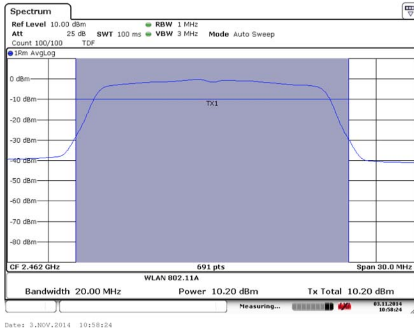
Fig. 30 Maximum Average Output Power (802.11g, Ch 11,36Mbps)
